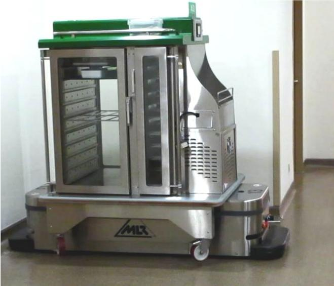
Figure15: Typical AGV with a supply trolley
